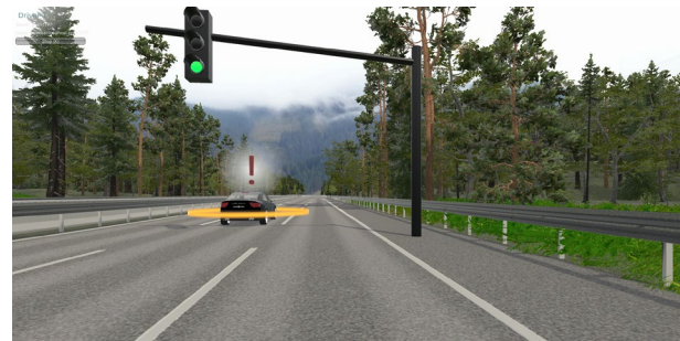
Figure 3. AR HUD. The vehicle with a distracted driver is visually highlighted on the windshield using augmented reality.
