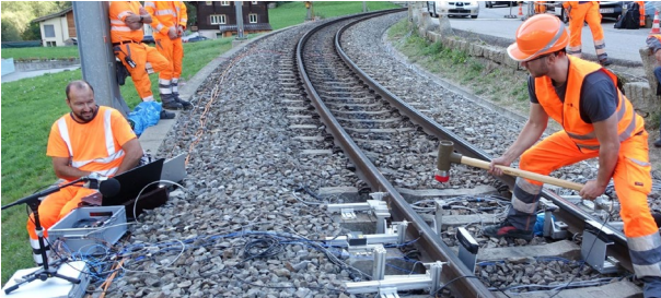
Figure 2: Impact hammer measurement to analyse the dynamic response of the track
